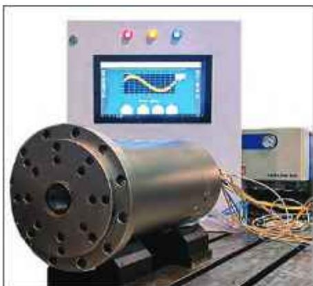
"i PreciSpindle\_18K" is an Instrumented, IIoT-enabled, integrated motor high-speed SMART spindle. The system is designed and developed in collaboration with M/s Acumac. It typically provides high precision and accuracy for machine tool applications. The developed "i PreciSpindle\_18K" comes with an edge device, IIoT gateway, dashboards, and decision boards for real-time condition monitoring, data analysis, and predictive maintenance. It is useful for both OEMs and Machine Tool Users.
