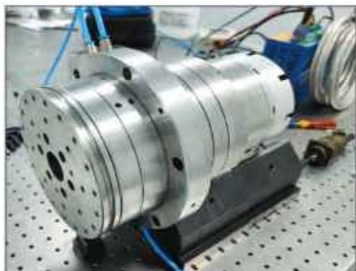
The project aims to develop an air bearing spindle with a porous air bearing restrictor. An air bearing for the spindle is most commonly used in precision machines when the accuracy requirements are high. Air bearing for spindle can be integrated into ultra-precision machine tools, metrology equipment like form testers & CMMs, etc, to achieve running accuracies.
