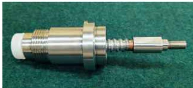
CMTI developed process technology for the machining of a 12 mm diameter, 5 mm pitch PS1 injection valve ball screw assembly. This assembly consists of ball screws, a ball nut, a sleeve, and a deflector, all featuring critical components with high dimensional and geometric tolerances ranging from 3 to 10 microns. The work was completed for LPSC ISRO Valiamala, and successfully delivered 156 sets during 2024-25.
