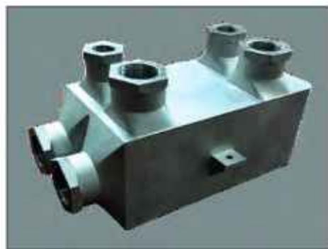
FCOC Heat exchanger printed by Laser based PBF process
