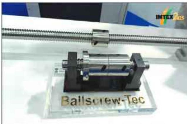
Recognizing this technology gap, CMTI has successfully designed and developed an internal deflector-type Ball Screw for precision machine tool applications, setting new benchmarks in indigenous manufacturing. This development aims to demonstrate advanced technology know-how and encourage domestic production of high-quality Ball Screws, reducing import dependency and strengthening India's manufacturing ecosystem.
