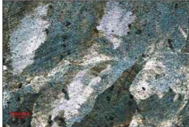
Microstructure of the printed test coupon
