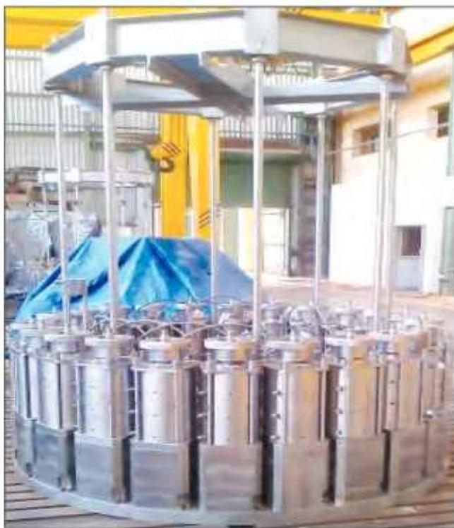
The CX-RPV is a specially designed tool for unseating the cover of the Reactor Pressure Vessel along with the copper seal from its installation. Similarly, the PFX-RPV is designed for unseating the pressing flange of the RPV from its installation
