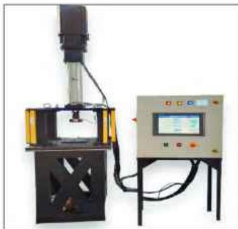
As part of a departmental initiative under the IAS, a 2-ton servo press capable of achieving 400 mm/s press speed was successfully designed and developed. The system is targeted toward precision forming applications.
