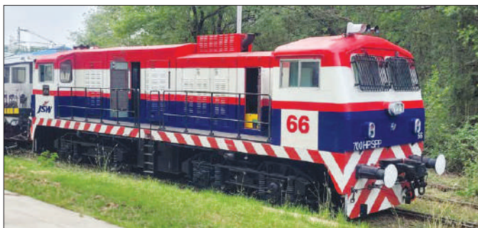
Designed & manufactured first-ever Dual Cab Diesel Electric Locomotive (700 HP rating) indigenously at BHEL, Jhansi
