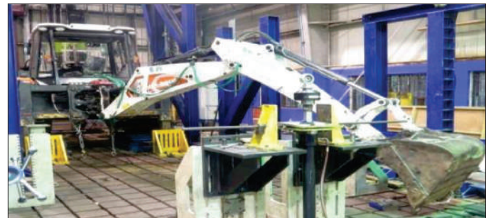
First time testing of Backhoe and Loader Lift Capacity in Fatigue Lab
