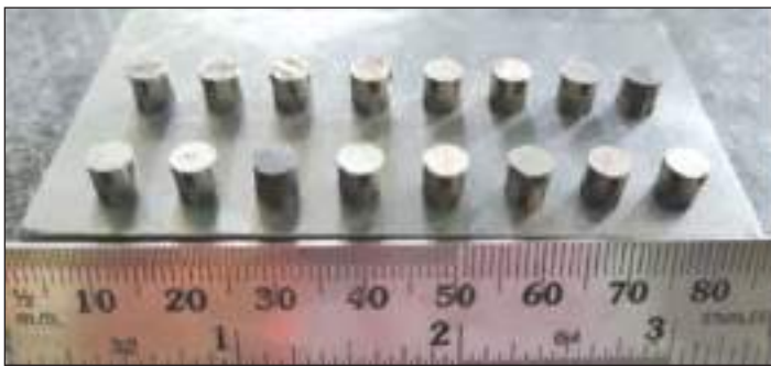
Bimetallic structures additive manufactured through DMD process
