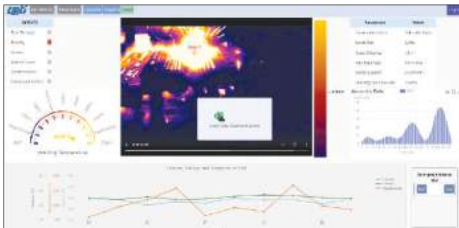
AI/ML based automated weld defect detection system
