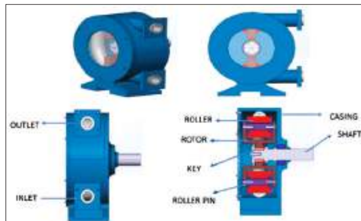
Hose pump assembly
