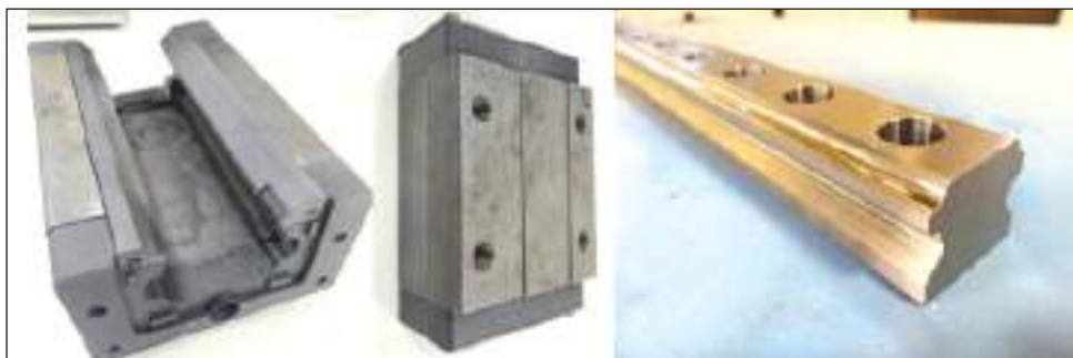
Operation rough machined LM guide block (with recirculation endcap) and rail
