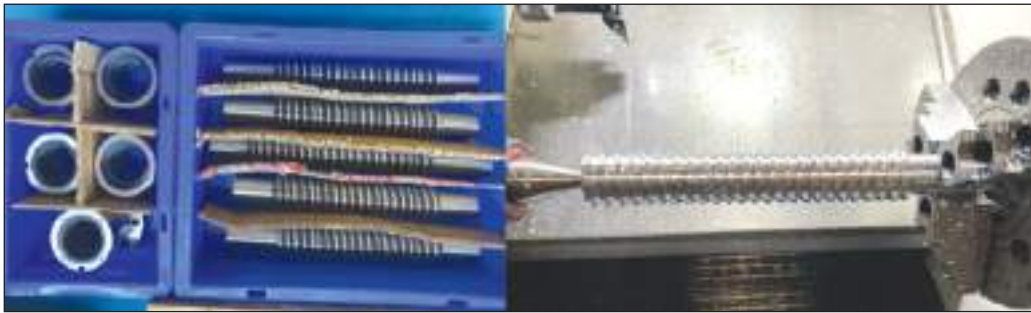
Ground Ballscrews & Ballnut, ready for thread grinding operation
