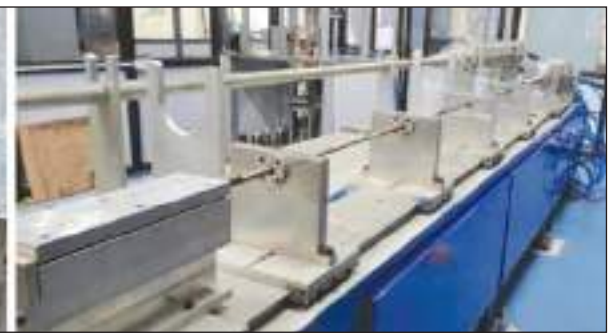
Testing of the bimetallic structures using split-hopkinson pressure bar set-up
