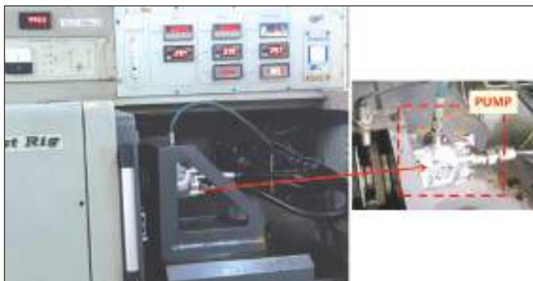
Engine driven hydraulic pump
