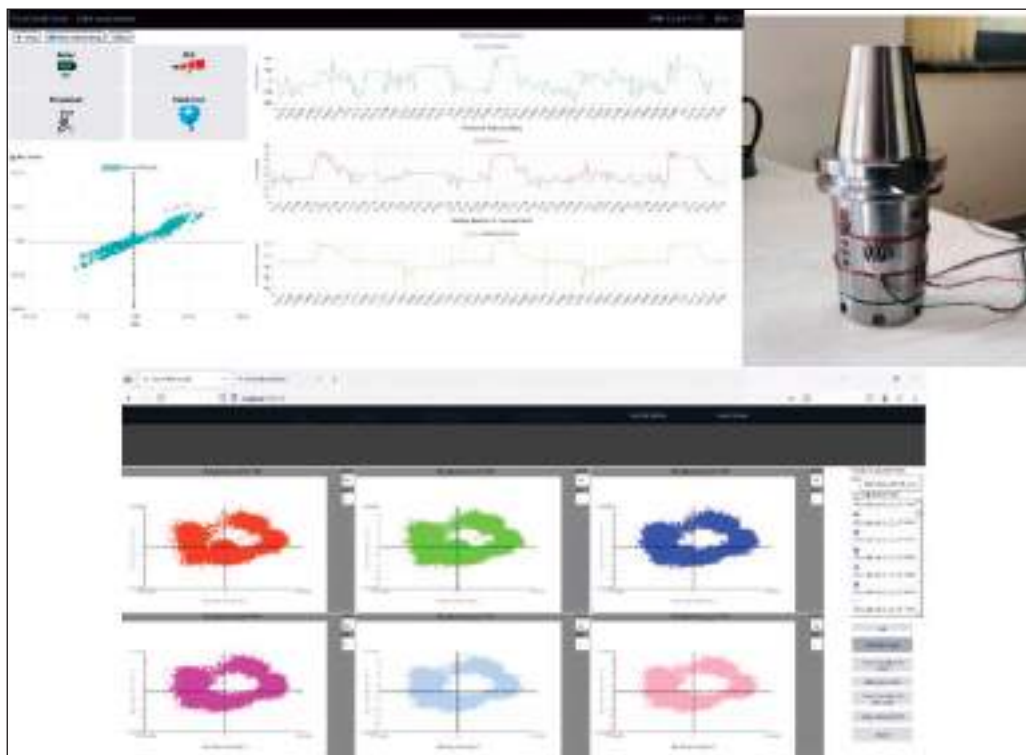
Digital twin with multi sensor integrated smart tool holder for cutting process monitoring
