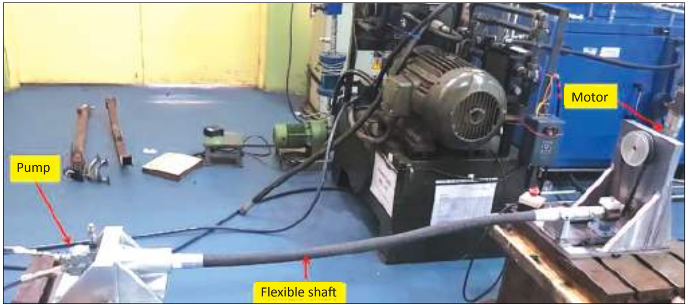
Vibration testing for hydraulic pump
