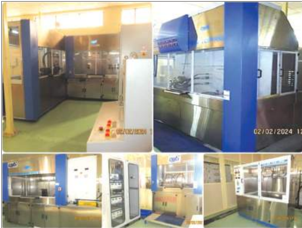
Hydraulic second line test rig
