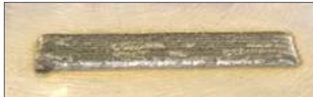
Inconel 625 part printed with developed facility
