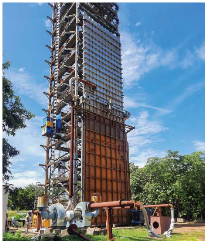
50 m tall testing stand for guillotine gates and dampers at BHEL Ranipet
