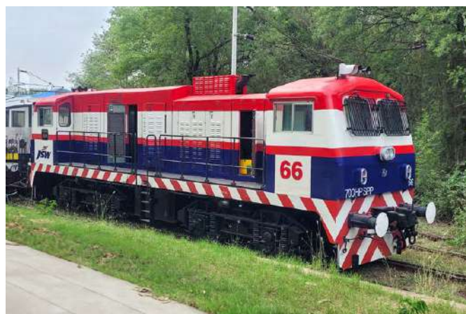
Designed & manufactured first-ever Dual Cab Diesel Electric Locomotive (700 HP rating) indigenously at BHEL, Jhansi
