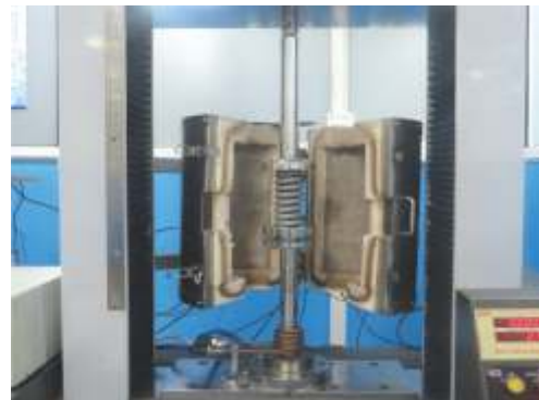
Load Relaxation Testing on Springs
