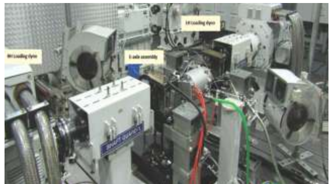
E-axle Performance and Durability Testing with 2 Dyno Setup
