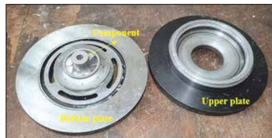
Component with developed work holding fixture
