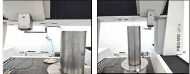
Inspection of Thin Cylinder
