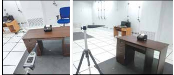
Noise Measurement of Dot Matrix Printer as per EU Norms
