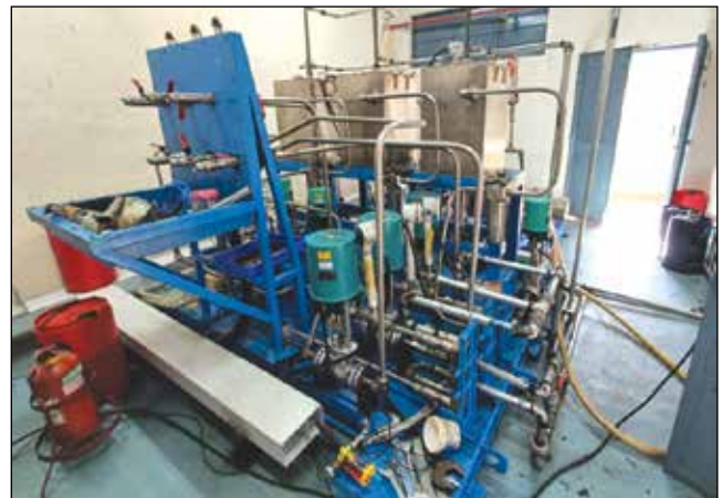
Thermal Performance Test Facility for Fuel Cooled Oil Cooler Heat Exchanger
