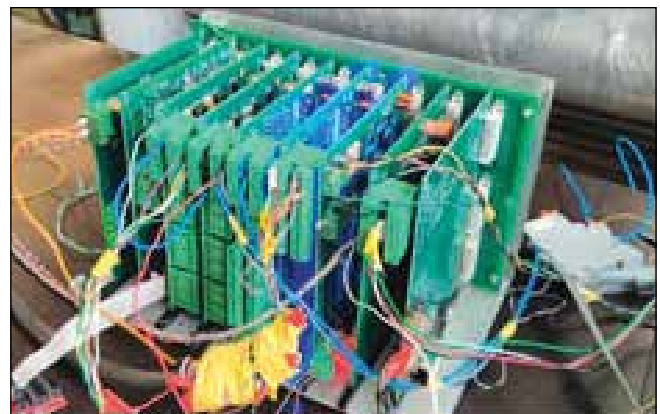
Micro-Controller Based Control System Interfaced To LR-450
