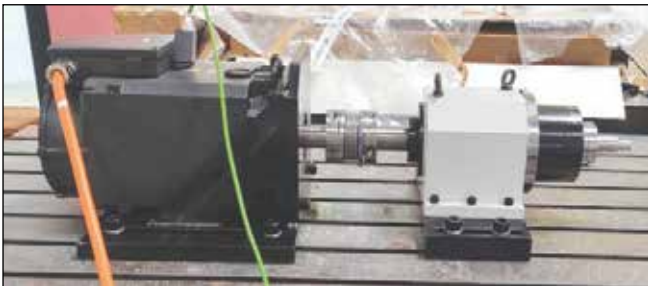
Assembly of Conventional Spindle Test Rig
