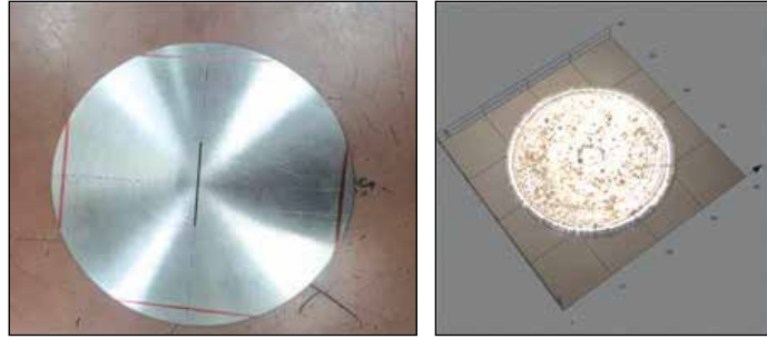
Ultrasonic reference block with Dia 0.4 mm Flat Bottom Hole machining
