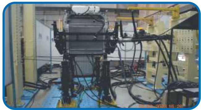
Multi-axial Durability Testing of Cooling Module Assembly
