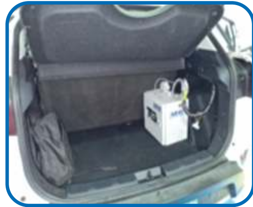
Controller Mounted in Vehicle Boot
