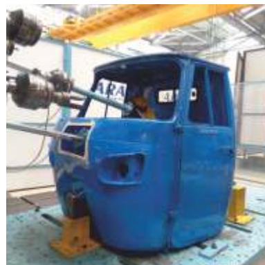
Seat Belt Anchorage Test on 3-wheeler
