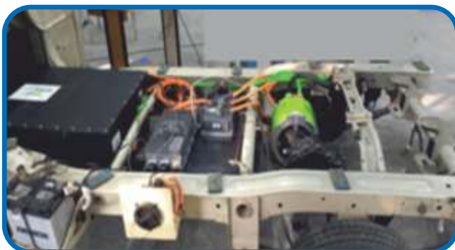
Developed E-axle fitted on 1.5T SCV
