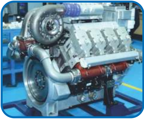
V-8, DI, Diesel 600 HP Engine for Defence Application
