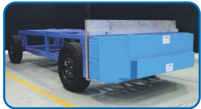
Mobile Barrier Trolley as per Euro-NCAP Protocol
