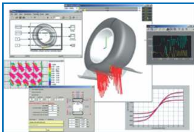
F-tire Model Fitting Process
