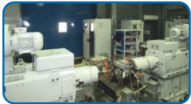
Machine-in-Loop setup for Vehicle Components Testing
