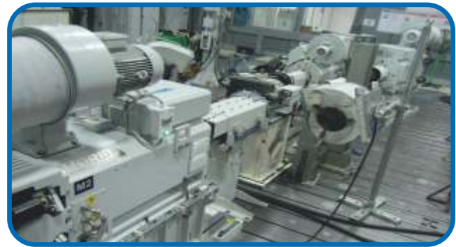
High Speed Test of EV Transaxle
