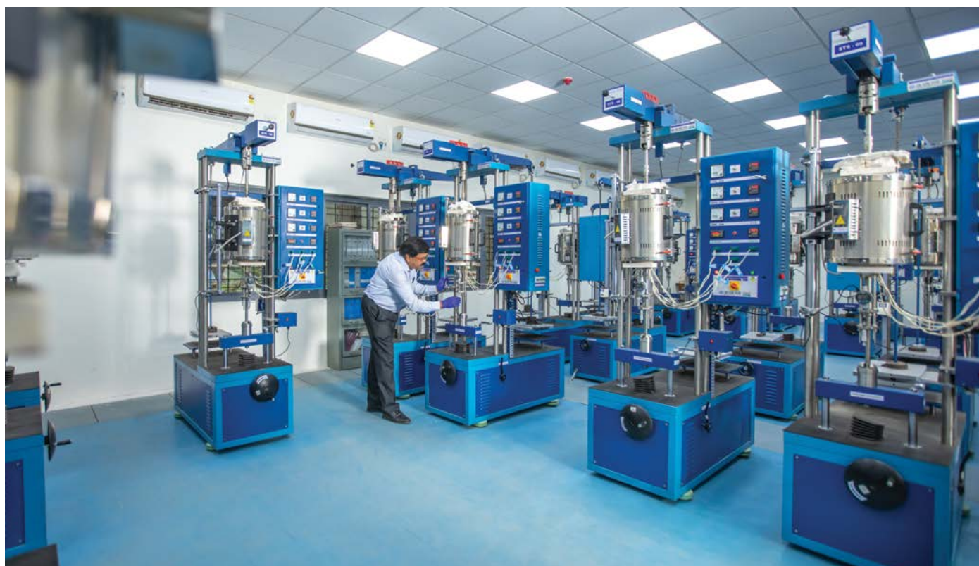
Creep testing facility for Advanced Materials at Metallurgy Department at Corporate R&D, Hyderabad
