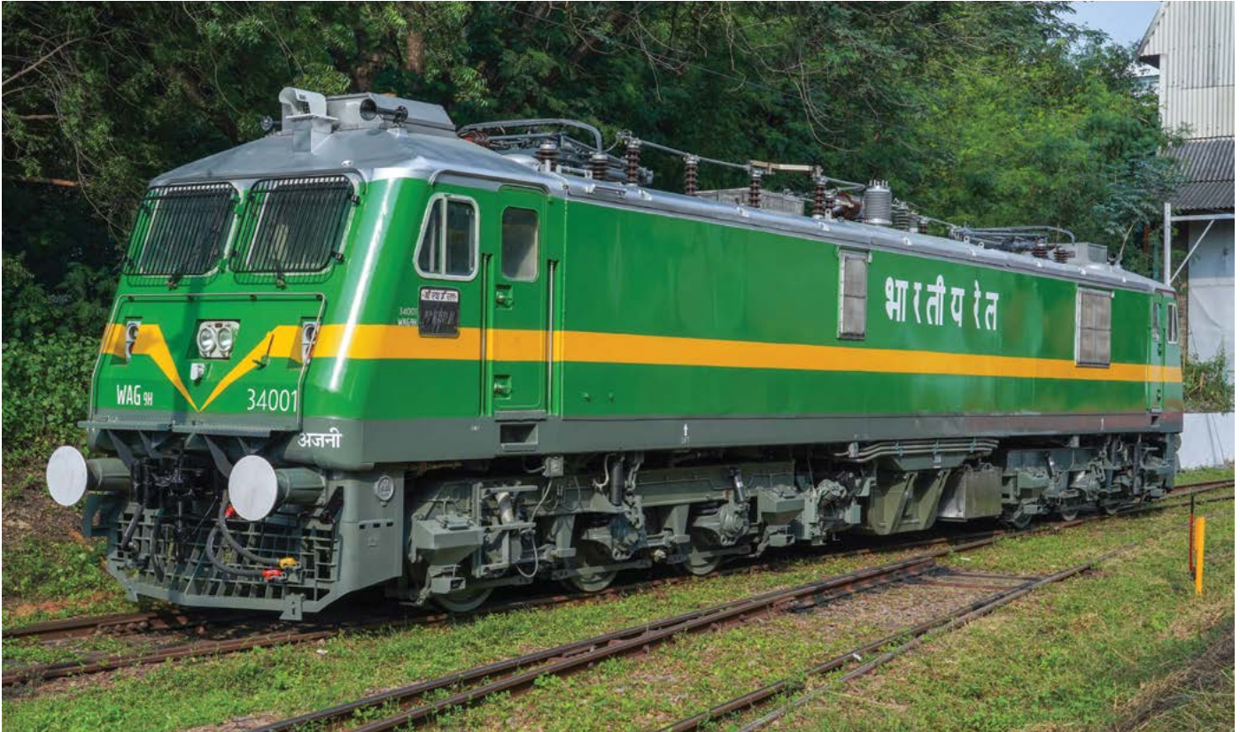
WAG-9H electric locomotive for Indian Railways supplied by BHEL
