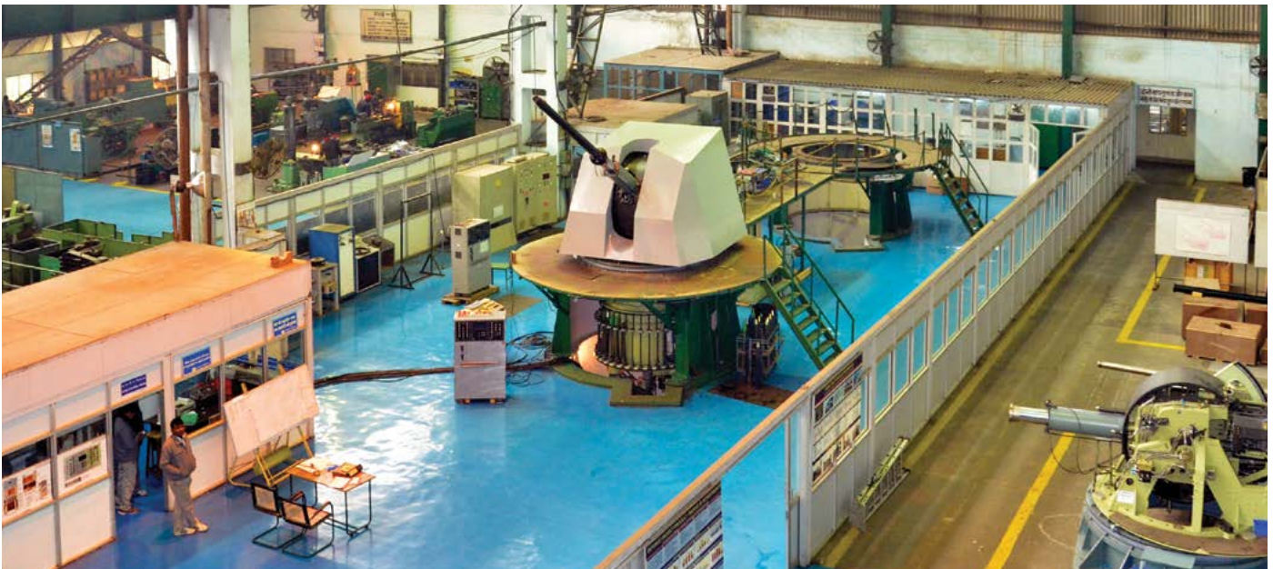
Super Rapid Gun Mount (SRGM) being manufacture at BHEL's Haridwar plant
