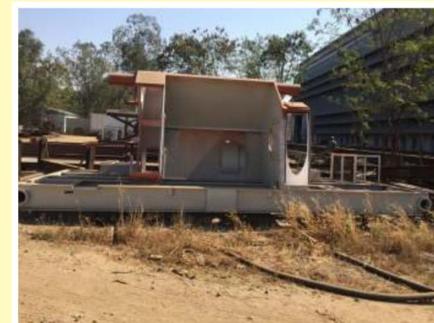
Drawworks Housing Equipment (Oiling Mast) -
