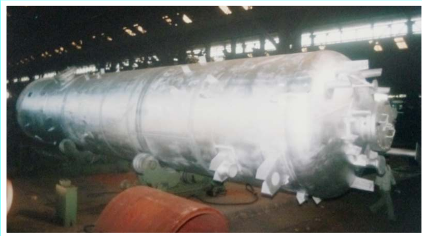
Item : Emergency H.P. Air Receiver Client : IOCL - PANIPAT- PREP PROJECT Item No. 36-V-513 Mfgd : at Byculla Unit Weight : 45.00 M.T.
