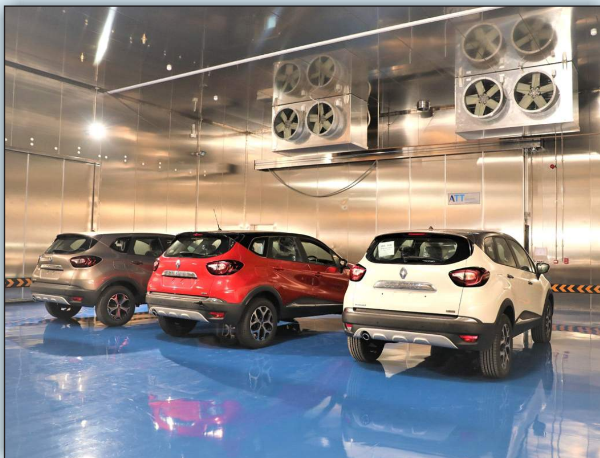
LOW TEMPERATURE SOAK ROOM AT GARC
