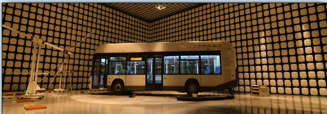
EMC FACILITY AT ICAT
