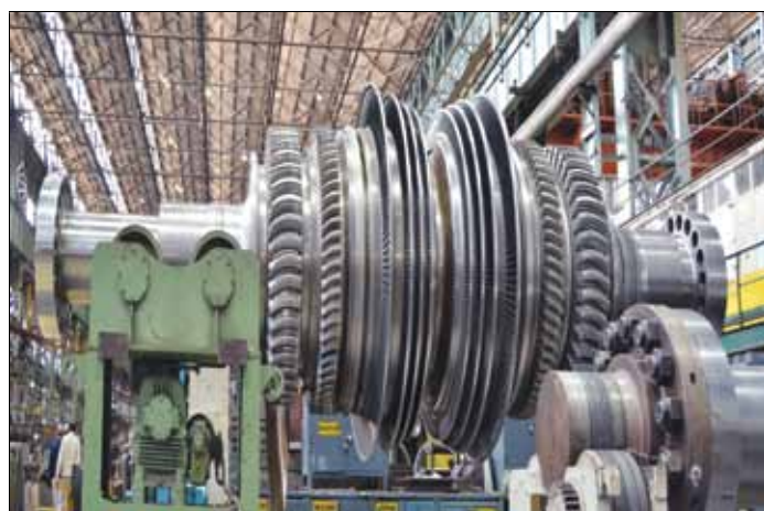
800 MW LP rotor under assembly at BHEL Hardwar
