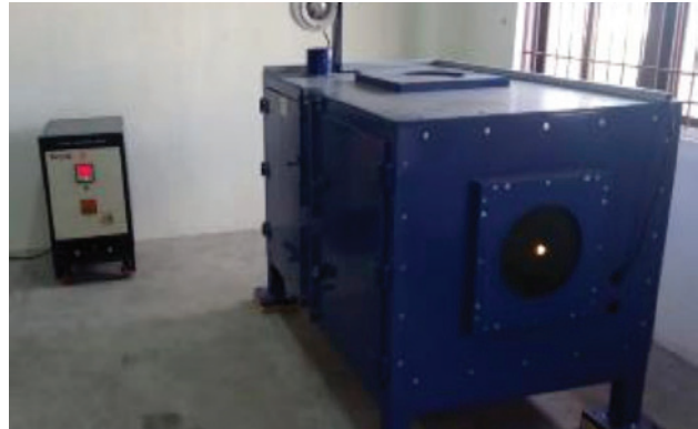
Battery – Destructive Testing
