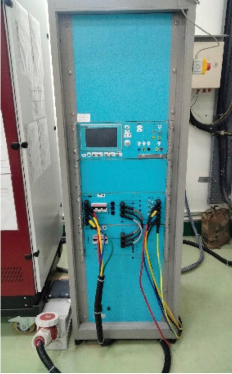
Test Setup for IEC 61000-4-34 (Voltage Dip, Interruptions and Variations)
