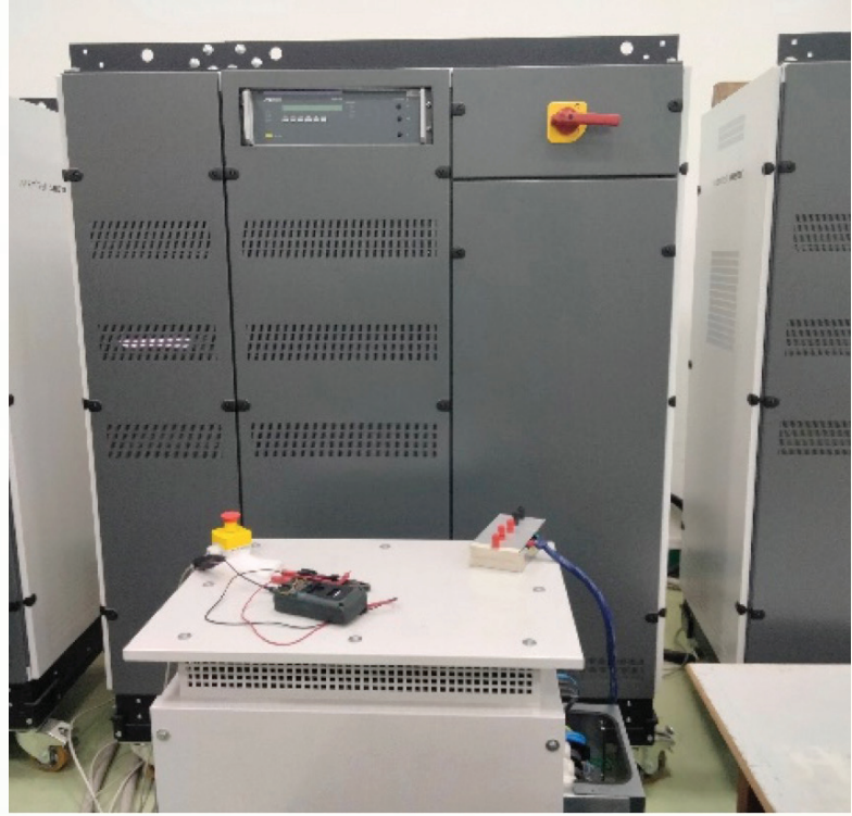
Test Setup for IEC 61000-2-2 (low frequency conducted disturbances)
