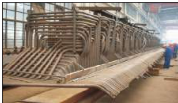
Burner Panel of Super-Critical Set for NTPC Barh 660 MW, being assembled at BHEL, Trichy Complex
