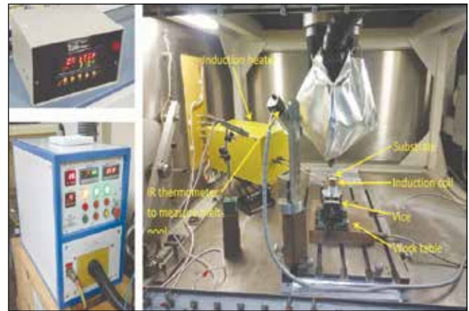
Induction-based substrate preheater with closed loop temperature control in DMD machine
