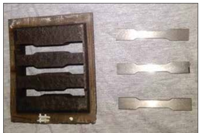
Tensile test specimens of 15-5 PH stainless steel by DMD process
