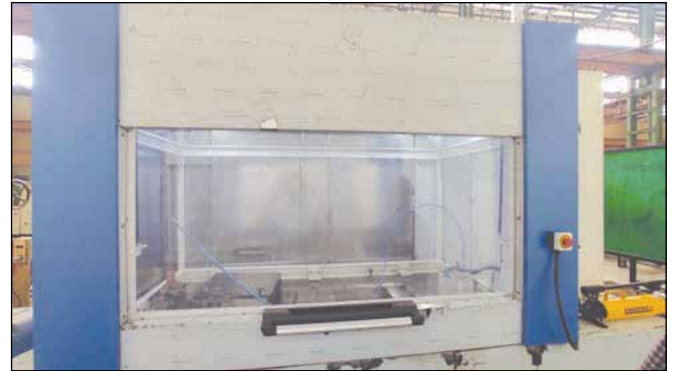
Static pressure test rig
