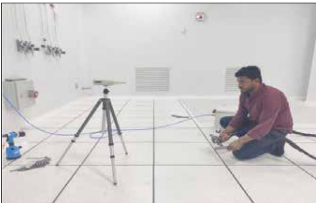
NVH testing and certification of hand held tools
