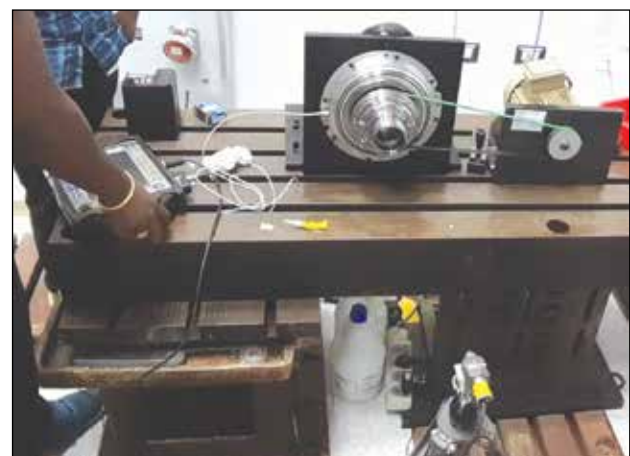
Dynamic balancing and vibration analysis of GE turbine rotor & turbine sub-assembly
