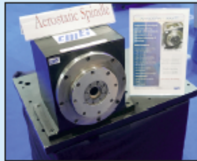
Ultra Precision Aerostatic bearing spindle
