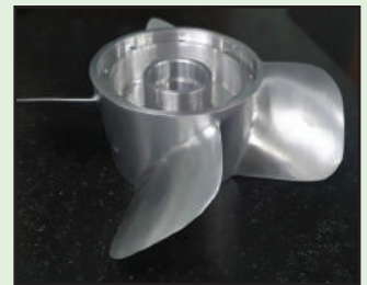
Machining of Propeller and Finished Propeller
