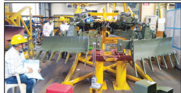
Onsite Calibration of Engineering Mine Flow Fixture for M/s L & T Pvt. Ltd. Bengaluru
