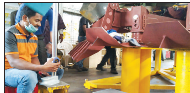
Onsite Measurement of Straightness and Parallelity of Machine Slides for M/s Mag India Industrial System Pvt. Ltd. Bengaluru
