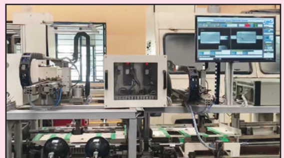
Fluted Roller Vision Inspection System has been commissioned in the production line
