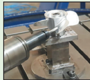
Machining of Propeller and Finished Propeller
