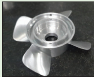
Machining of Propeller and Finished Propeller
