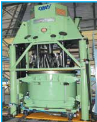
Vertical Planetary Mixer (MY-300) Capacity : 5000 kg
