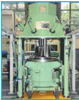
Vertical Planetary Mixer (MY-16) Capacity : 400 kg
