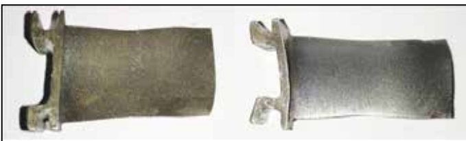
Aero Engine Blade (Before & After AFFM Process)
