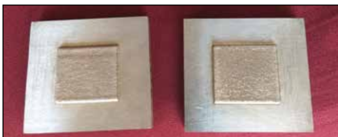
Colmonoy-5 alloy coating on SS316LN through DMD process
