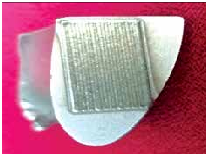
Single-layer deposition of Inconel-625 through DMD process
