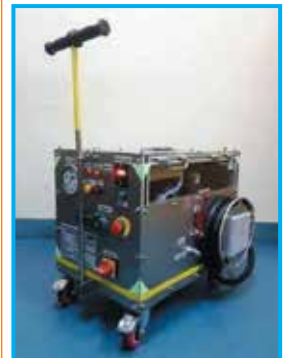
Battery Operated Hydraulic Power Pack to Charge Fighter Aircraft Brake Accumulator
