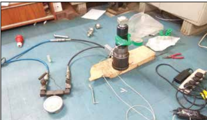
Vibration Measurement of handheld Riveted Tool used in Railways
