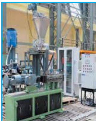
Twin Screw Continuous Mixer (TSCM-3) Capacity : 40-100 kg
