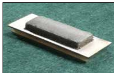
SS316L printed through the DMD process on DMLS - built parts
