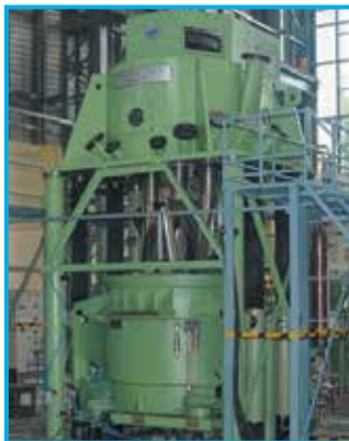
Vertical Planetary Mixer (VM-4.5T) Capacity : 4500 kg
