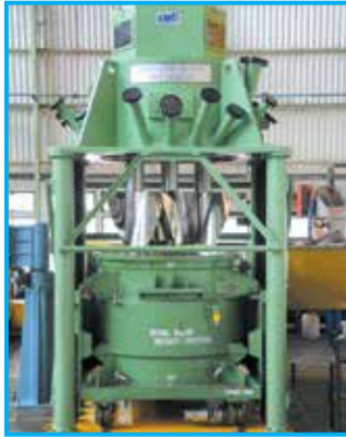
Vertical Planetary Mixer (VM-1000) Capacity : 2500 kg
