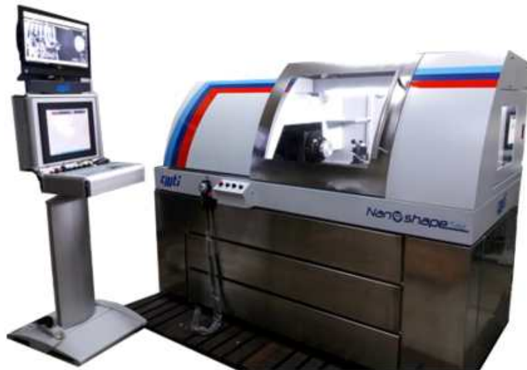
Precision and Highly Stiff Diamond Turning Machine
