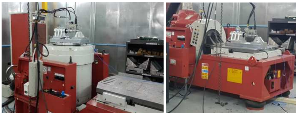
LESA Qual Model under vibration test
