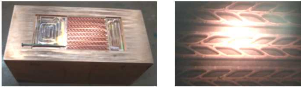
Micro Channels made in Copper
