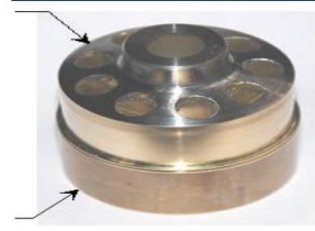
Bi-metallic parts deposition (Steel on Al-Bronze) by DMD
