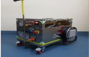
Battery operated hydraulic system to charge parking brake accumulator of aircraft
