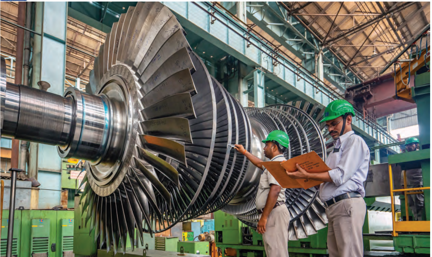
800 MW LP turbine under inspection at New Turbine Shop in BHEL Haridwar
