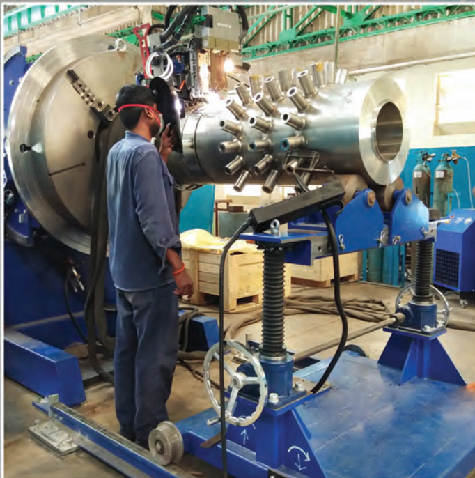
End Cover Welding for the Super Heater Header for 800 MW - AUSC
