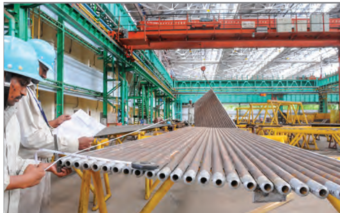
Spiral Water wall assembly for supercritical boilers in progress at BHEL, Tiruchirappalli
