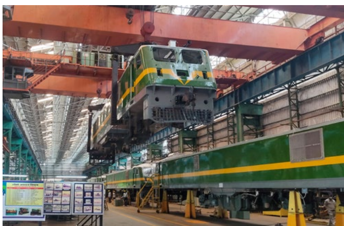
WAG 9H locomotives under manufacture for Indian Railways at TP, Jhansi
