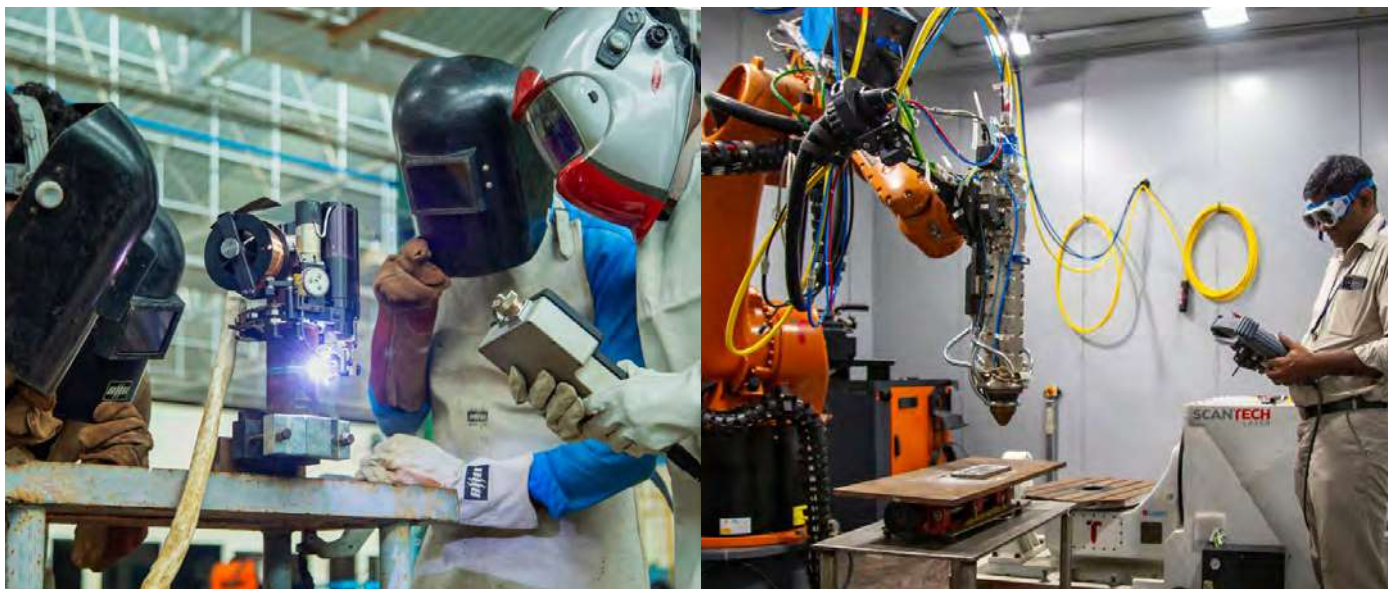
Orbital testing machine test setup (left) and robotic arm laser welding setup (right) at Welding Research Institute, BHEL Tiruchirapalli
