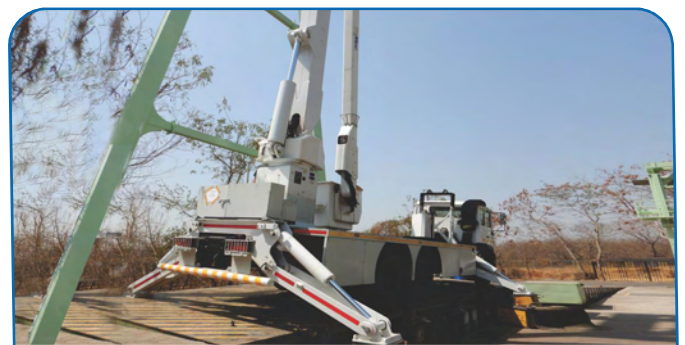
Tilt Stability Test for Truck mounted Boom Crane
