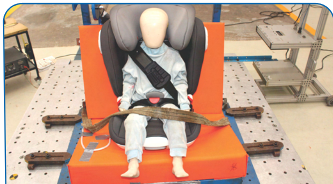
NABL Accreditation for Child Restraint System Testing and Approval as per AIS072 and ECE R44.04
