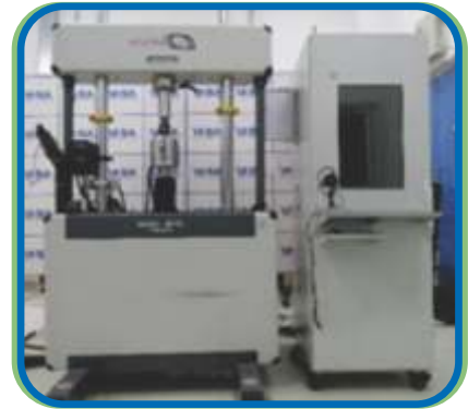
Servo Hydraulic Test System for Fatigue Characterization
