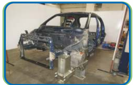
Experimental Modal Analysis and Dynamic Stiffness Evaluation for BIW Structure
