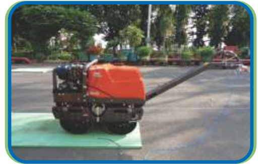
Noise & Vibration Measurement on Hand Held Road Roller
