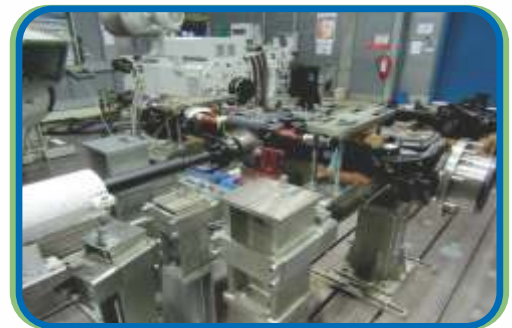
Setup for Axle Power Loss Analysis
