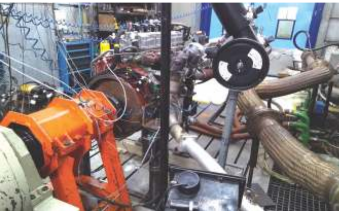
◀ 6 cylinder TCIC CNG Engine Setup ▶
