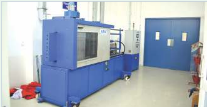
◀ Battery Abuse Testing Machine ▶
