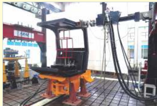
◀ Long Stroke Actuator for ROPS Test Facility ▶
