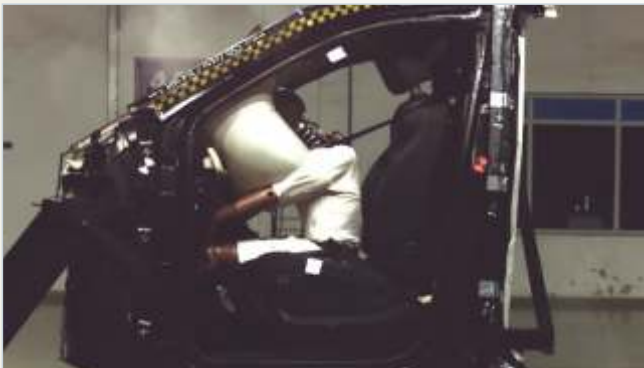
Interior Fittings evaluation as per UNECE R21
