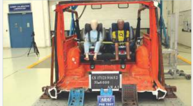
Validation Testing of Seats as per ADR 34
