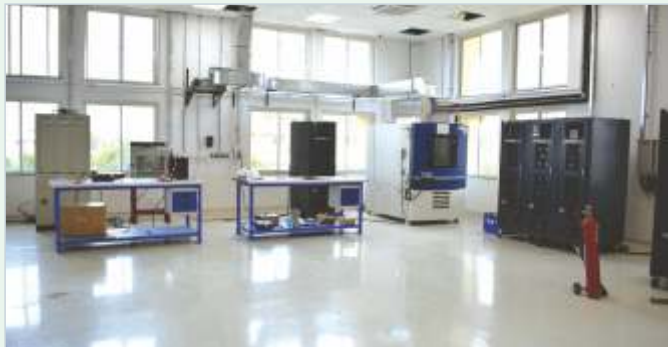
◀ Battery Cell Tester with Temperature Chamber ▶
