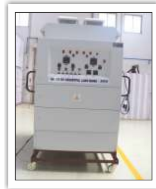
High Voltage EV Discharge Unit
