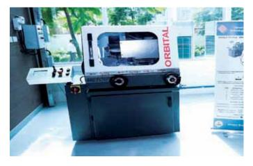
Orbital Motion Abrasive Cutting Machine developed by Centre of Excellence at IIT, Madras
