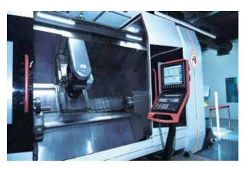
5-axis Multi Tasking machine developed by Centre of Excellence at IIT, Madras
