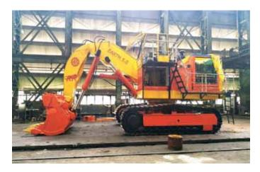
5 Cubic Meter Hydraulic Excavator - HEX 400 developed by Centre of Excellence at HEC Ranchi
