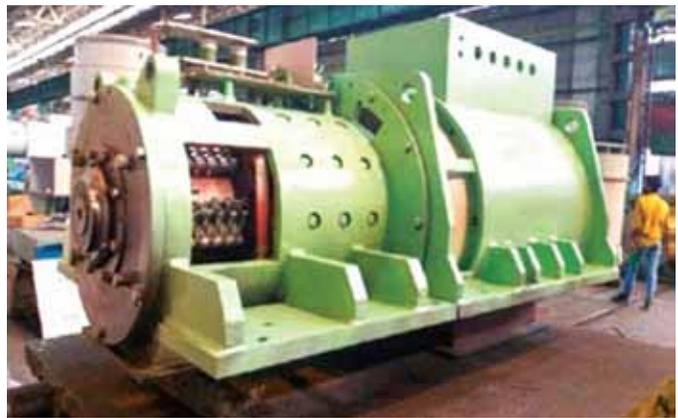
500kW Main Motor Generator (MMG) (assembly of AC & DC machine) for defence application designed & manufactured by BHEL
