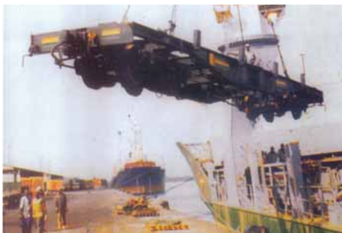
Container Flat wagons exported by the Company being unloaded at Port Autonome d' Abidjan.
