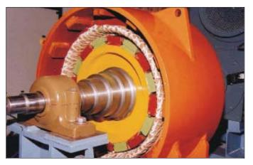
38 kW, 220 Volts, 400 Hz Compact Permanent Magnet Generator (PMG) suitable as pilot exciter for 250 MW TG developed in-house at BHEL
