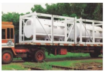
Super Insulated Skid mounted Cryogenic Tanks by BHPV.
