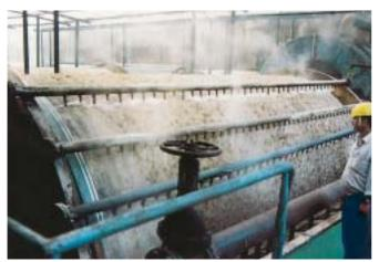
Pulp mill washers at Cachar Paper Mill of HPC.
