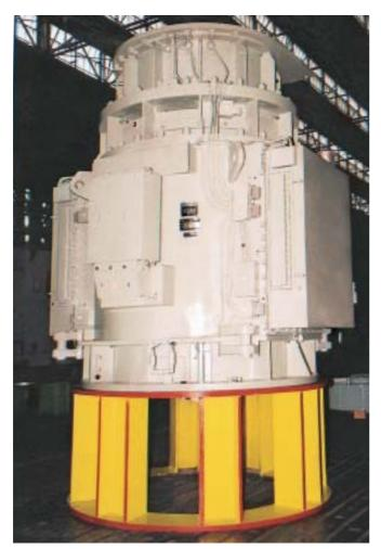
Largest capacity (6MW, 1500 RPM, 6.6KV) Vertical motor produced by BHEL.
