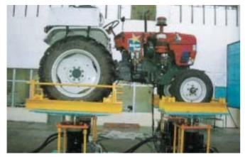
Testing at ARAI, Pune for structural evaluation of all sheet metal components in Tractors.
