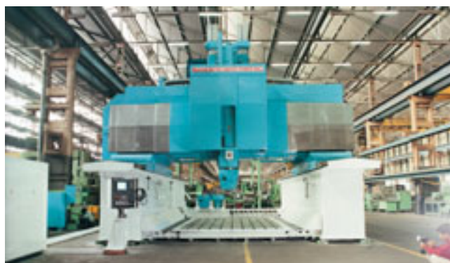
High technology Five Axis Gantry Power Mill, designed and manufactured by HMT
