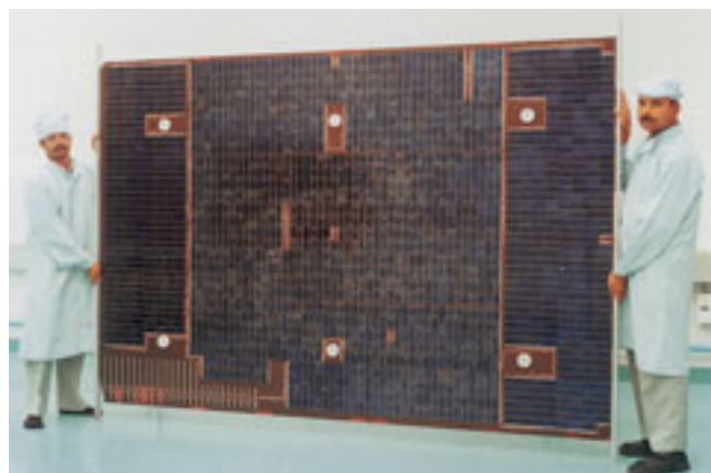
First Space-grade solar panel assembled at BHEL, Bangalore for satellite application for ISRO
