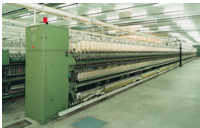
Ring Frame LR6 AX, with Auto Doffer 1200 Spindles, being manufactured by Lakshmi Machine Works
